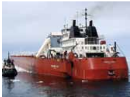
Presque Isle , the second 1,000-foot lake freighter, is an integrated tug-barge design. Also note smaller tug on its port side.
