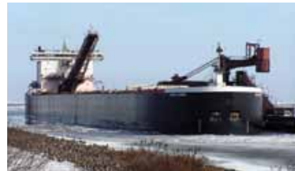
The Burns Harbor , built in Sturgeon Bay, Wisc. Its wide, overhanging bridge with widely placed stacks and non-flared bow are characteristic of Sturgeon Bay-built freighters.
